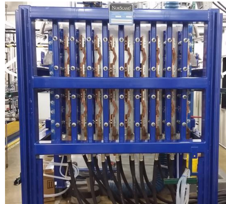
Cells are duplicated into a single stack
